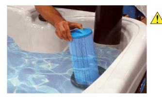
Make sure the filter has soaked at least 30 minutes before you install it. Insert the filter all the way and screw it in. Do not over-torque the cartridge during installation, just hand tighten gently.
