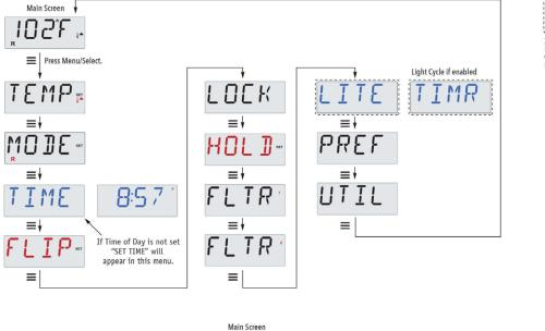
Waiting a few seconds in the Main Menu will allow the display to revert to the Main Screen. Most changes are not saved unless Menu/Select ≡ is pressed. Refer to key above.
