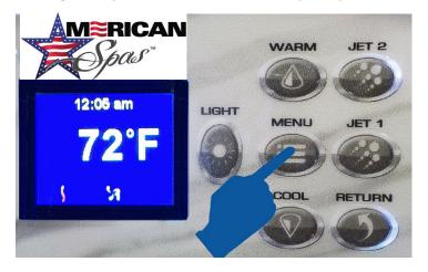
This time select Filter Cycles. (Press the MENU button to access the sub-menus.)
