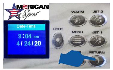
Once the screen has reverted back to temperature, you can now adjust Filter Cycles. **NOTE: You do not necessarily have to adjust the Filter Cycles because the default factory settings give you two Filter Cycles per day automatically.** In any case, to access the Filter Cycles, press the MENU button.
